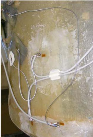
**Fig. 8.** Strain gauges on the tank
